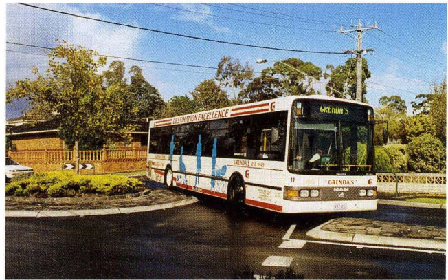
Front bus overhang over traffic island at roundabout
