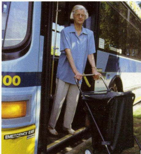
Lower bus floor provides improved access for bus patrons, particularly the elderly and people with disabilities.
