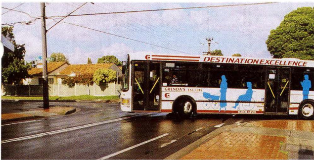
Bus encroaching over road centreline
